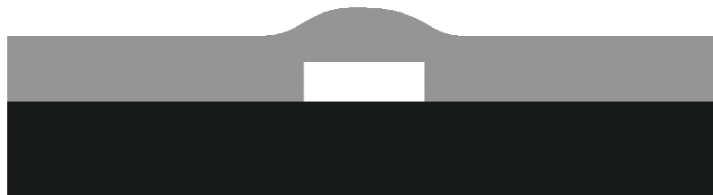
Figure 4.5: Schematic representation of layer variations around a ridge waveguide
