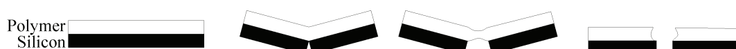
Figure 4.11: Schematic representation of four steps in cleaving a silicon wafer with polymer layer stack
